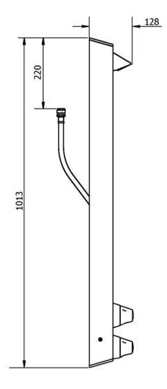
The T105BLR shower panel is pre-plumbed with an integral dual control Type 3 approved thermostatic mixing valve, which features:
