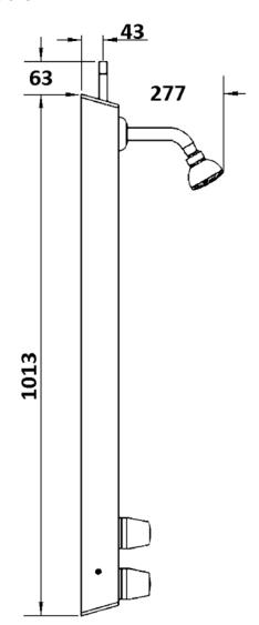
The T106A shower panel is pre-plumbed with an integral Type 3 and WRAS approved thermostatic mixing valve, which features:
