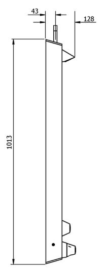
The T113ALR shower panel is pre-plumbed with an integral thermostatic mixing valve, which features:
