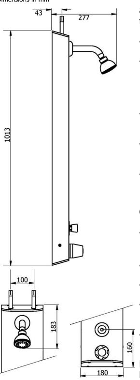
The T206A shower panel is pre-plumbed with an integral thermostatic mixing valve, which features:
