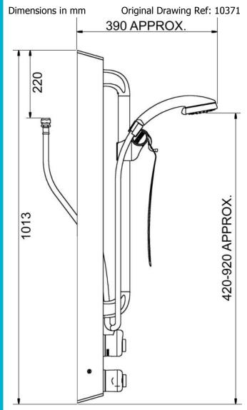
The **T107B2L** shower panel is pre-plumbed with an integral dual control Type 3 approved thermostatic mixing valve, which features:
