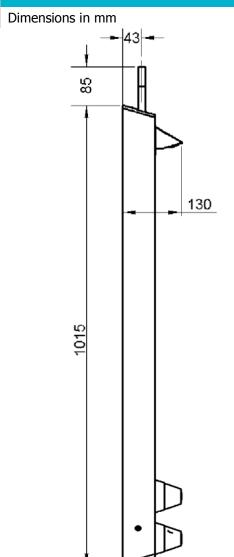
The T105ALR shower panel is pre-plumbed with an integral dual control Type 3 approved thermostatic mixing valve, which features:
