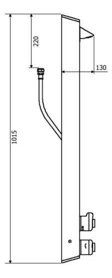
The T105B2L shower panel is pre-plumbed with an integral dual control Type 3 approved thermostatic shower valve, which features:
