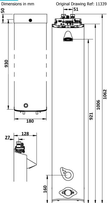
TOTAL HEIGHT OF PANEL + PIPECOVER = 1006 + 2 + 930 + 50 - (OVERLAP) - OVERLAP IS VARIABLE, 20-40MM - 930 LENGTH CAN BE CUT TO SUIT
