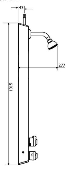
The T106A2L shower panel is pre-plumbed with an integral Type 3 and WRAS approved thermostatic mixing valve, which features:
