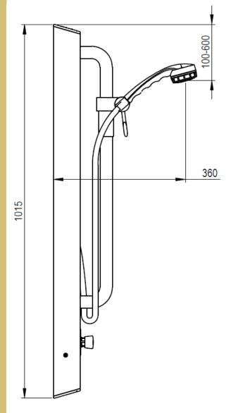
The T307B shower panel is pre-plumbed with an integral Type 3 approved thermo-static mixing valve, which features:
