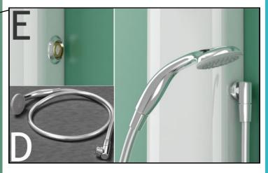
**Assisted mode:** For able and non ablebodied users who require assistance or supervision during showering. In this mode the carer/supervisor attaches the handset and hose (D) by screwing the hose connector into the ligature and vandal resistant outlet fitting (E) on the side of the panel. Water is <u>automatically</u> diverted to the handset on opening the shower flow control (B). The water temperature (C) is adjusted in the usual way.
