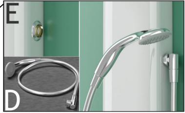
**Assisted mode:** For able and non ablebodied users who require assistance or supervision during showering. In this mode the carer/supervisor attaches the handset and hose (D) by screwing the hose connector into the outlet fitting (E) on the side of the panel. Water is <u>automatically</u> diverted to the handset on opening the single lever flow control (B). The water temperature (C) is adjusted using the 360° rotation double lever.
