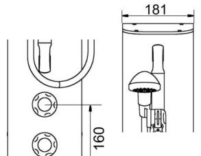
Original Drawing Ref: 10341 The **T1Y8B** shower panel is pre-plumbed with an integral dual control Type 3 approved thermostatic mixing valve, which features:
